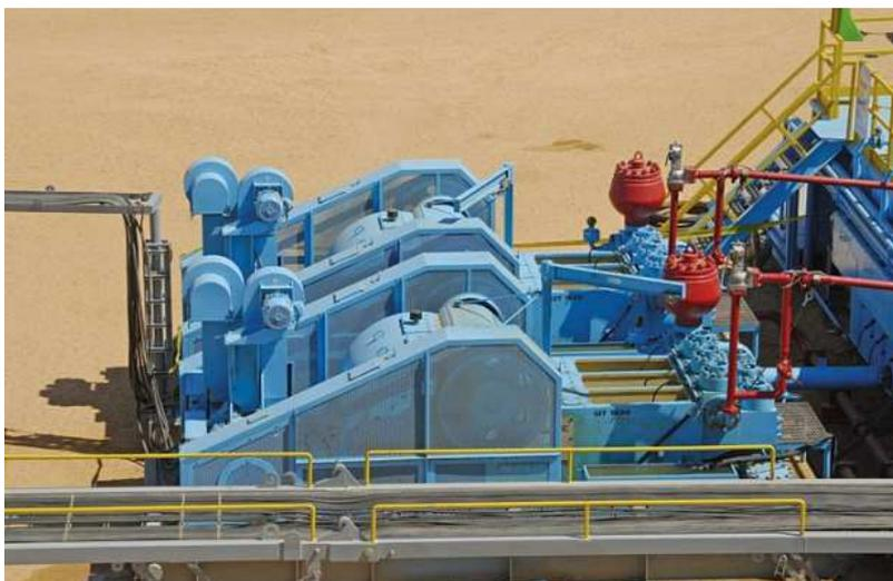
Mud pumps are the “heart” of a rig. They circulate mud and control well hydraulics. Piston types can be duplex (two double-acting cylinders) when flow/pressure is modest or triplex (three-acting cylinders) for large flow demands, typically for deeper drilling.
