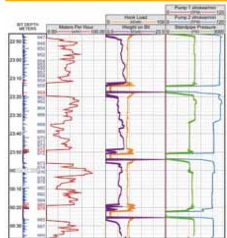
Figure 7. Drilling log (constant wob) - HH102.
