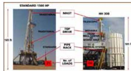
Figure 4, Comparison between conventional 1500HP rig and HH300 rig features.
