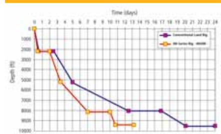
Figure 8. Performance comparison between average of conventional rigs and new HH200 rig.
